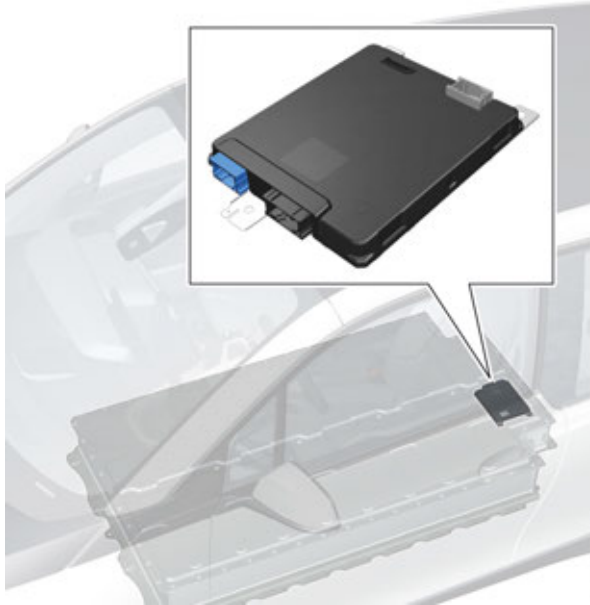
Battery management electronics
